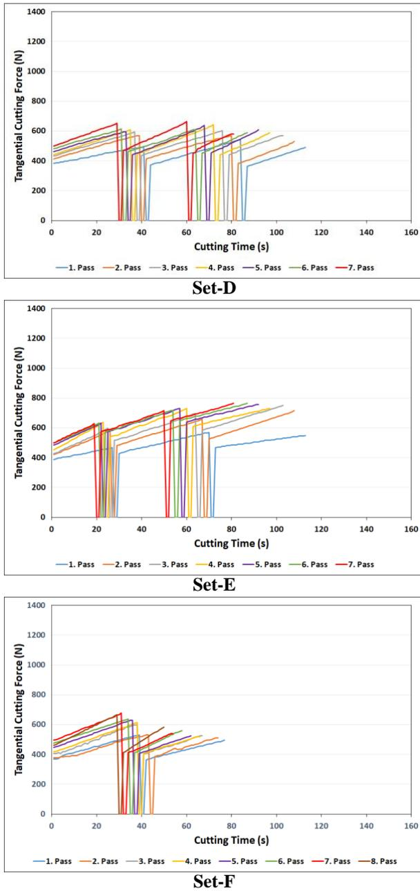
Figure 4. Evolution of the Tangential Cutting Force
