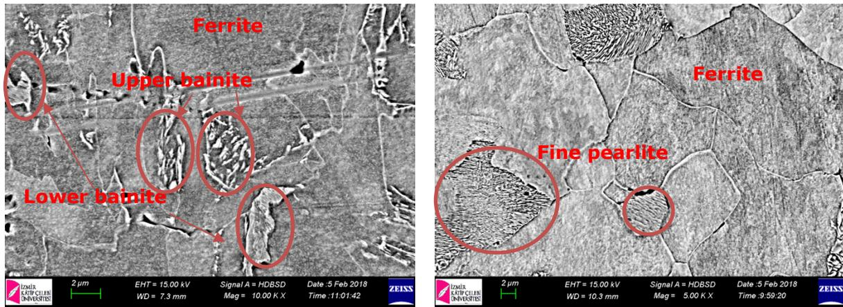
(a) Accelerated Air Cooling (AAC) (b) Accelerated Air Cooling plus Normalization (AAC-N)
