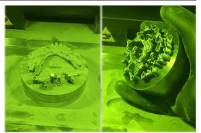
Fig.13 LMF - Laser Metal Fusion technology
