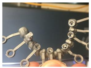
Fig.17. The milled and finished dental framework
