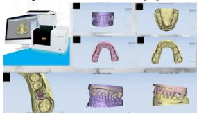
Fig.10. Optical scannig of inpalnt based dental restaurations
