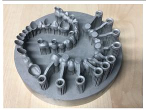
Fig.15. Printed, heat-treated, sandblasted platform
