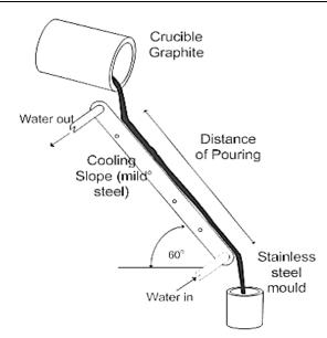
Figure 4. Schematic of cooling slope method [4].
