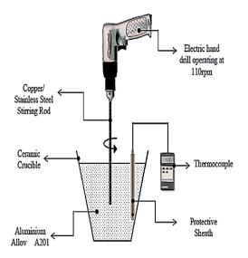
Figure 2. Schematic of Semi-Solid Rheocasting [3].
