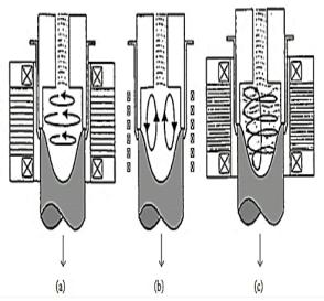
**Figure 3.** Schematic diagram of dissimilar flow modes: (a) horizontal agitation, (b) vertical agitation and (c) helical agitation [4].
