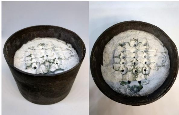
Fig. 5: Cracked embedding material
