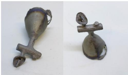
Fig. 6: Workpiece with argon gas generated casting cavities
