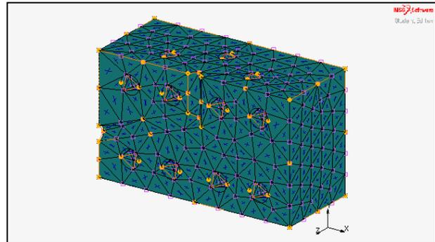
Fig. 2. Finite element mesh of the 3D modelled extrusion die.
